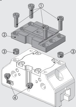
Unscrew the 4 screws ①, remove the plate ② and pull out the centring rings ③. Then unscrew the 2 plugs ④.
