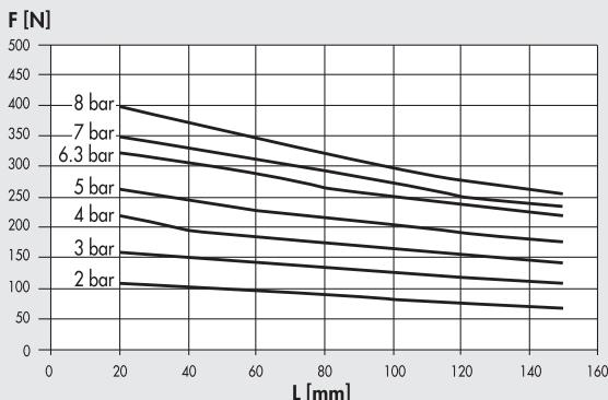
\*\*\* Referred to a single jaw. The total force is obtained by multiplying the value by 2.
