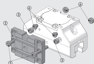
Replace the 2 plugs ④ on the opposite side of the gripper and insert the 2 centring rings ③. Position the plate ② and the two long screws ⑤ (supplied with the gripper). On the opposite side of the plate, insert the two nuts with a screwdriver slot ⑥ (supplied with the gripper) and tighten them against the screws ⑤.
