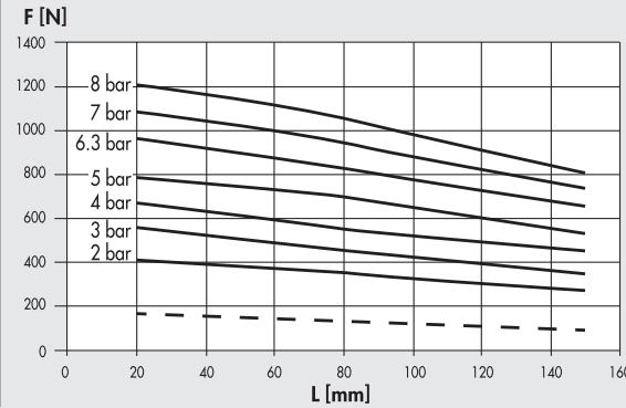
\*\*\* Referred to a single jaw. The total force is obtained by multiplying the value by 2.
