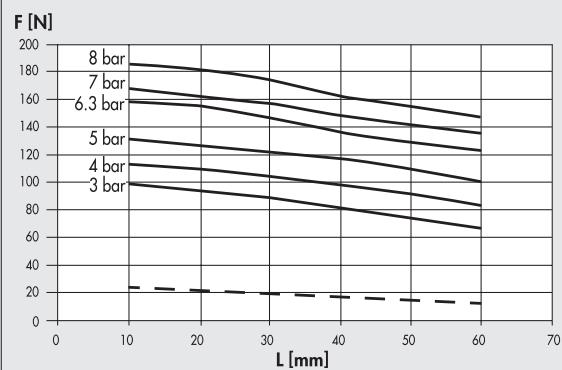
\*\*\* Referred to a single jaw. The total force is obtained by multiplying the value by 3.
