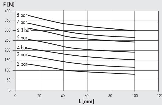
\*\*\* Referred to a single jaw. The total force is obtained by multiplying the value by 3.
